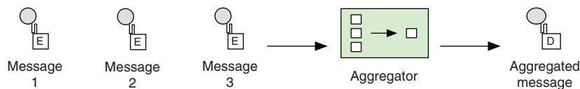
Figure 8.2 The Aggregator stores incoming messages until it receives a complete set of related messages. Then the Aggregator publishes a single message distilled from the individual messages.
