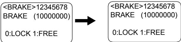
4) Hold the deadman switch (on the back of the T/B). Then hold down the [MOVE] key and press the [+X] key continuously to release the brake of the specified axis only while the keys are pressed. The brakes will activate when the [MOVE] key or [+X] key is released.
