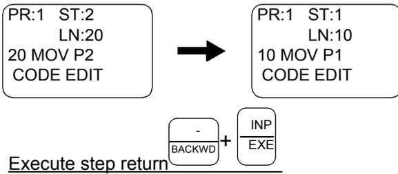
2) While holding down the [BACKWD] key, hold down the [EXE] key. The robot will start step return.
