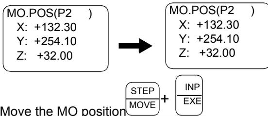
2) When the [EXE] key is pressed while holding down the [MOVE] key, the robot will move with joint interpolation to the currently displayed position data place only while the [EXE] key is held down.
