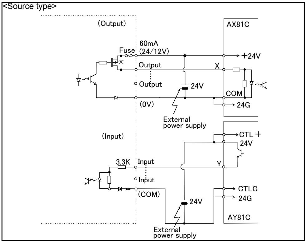
Fig.9-2:Connection with a Mitsubishi PLC (Example of source type)
