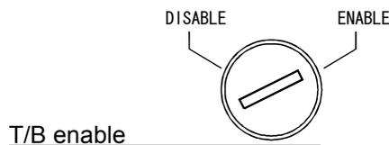
2) Set the T/B [ENABLE/DISABLE] switch to "ENABLE".
