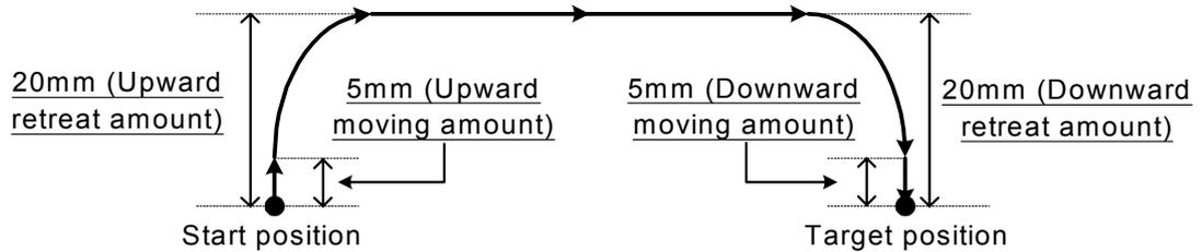
\*If Z is different between the movement starting position and the target position, it will operate as follows:
