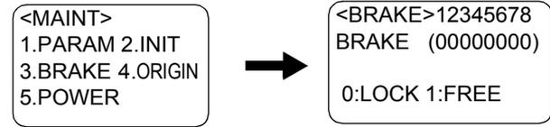
2) Press the [3] key, and select the brake release screen.
