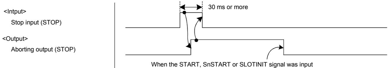
(8) STOPSTS (Output during stop signal input)
