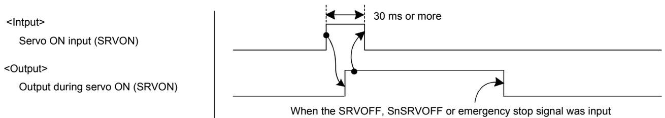
(12) SRVOFF (Servo OFF input/servo ON disable output)
