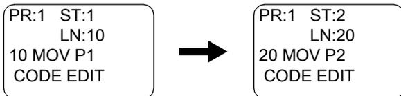
2) While holding down the [FORWD] key or [STEP] key, hold down the [EXE] key. The robot will start moving.
