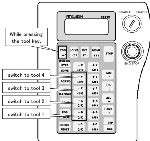
Set the tool data you want to use in the MEXTL1 to 4 parameters, and select the number of the tool you want to use according to the following operation.
