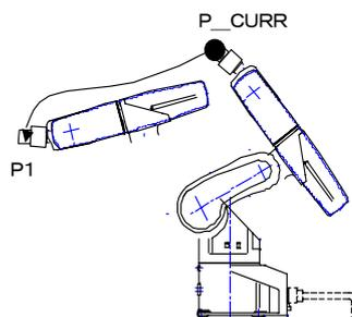
Fig.4-9: Example of joint interpolation motion path
