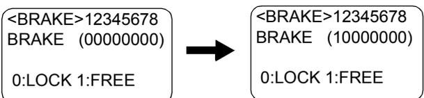
3) Press the [1] key to change the number corresponding to the axis for which the brakes are to be released to 1. Refer to [Table 3-5](#) and set the axis designation. In the example on the left, the J1 axis brake release is designated for the RP-1AH.
