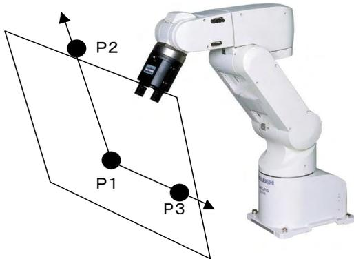
As can be seen in the diagram to the left, any plane can be defined by three points (P1, P2, and P3), after which an evaluation of which side of the plane it is in (the side that includes the robot origin or the other side) can be performed.
