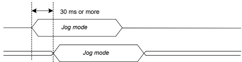
(Replies the setting value of the jog mode input signal with jog mode output.)
