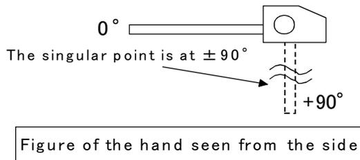
The singular points are when the wrist axis J5 is at +90 degrees, and when the center of axis J6 is located at the origin and the wrist is facing upward. In these cases, axes J1 and J5 are located on the same axis and it is not possible to calculate the robot position.
